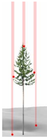
Figure 2. Schematic showing multiple LIDAR returns resulting from the laser light being only partially obstructed by tree branches.
