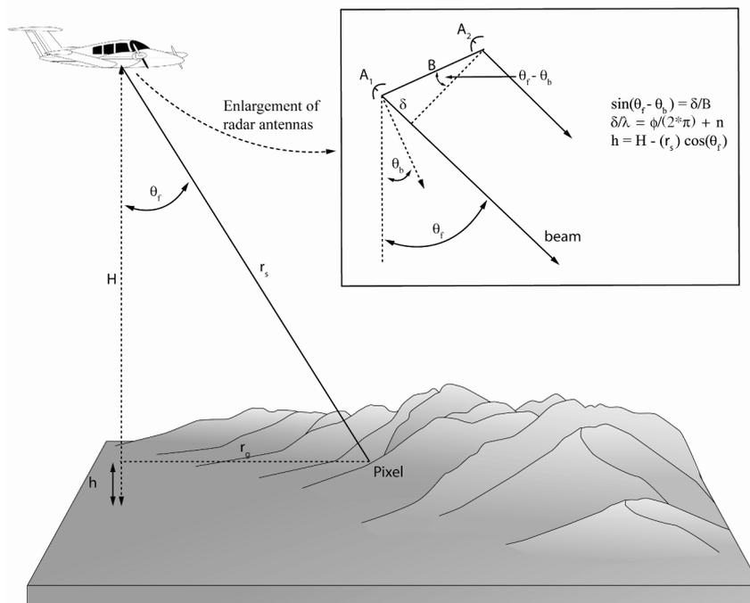
Figure 3-10. Geometry of RADAR interferometry. Adapted from Mercer (2004).
