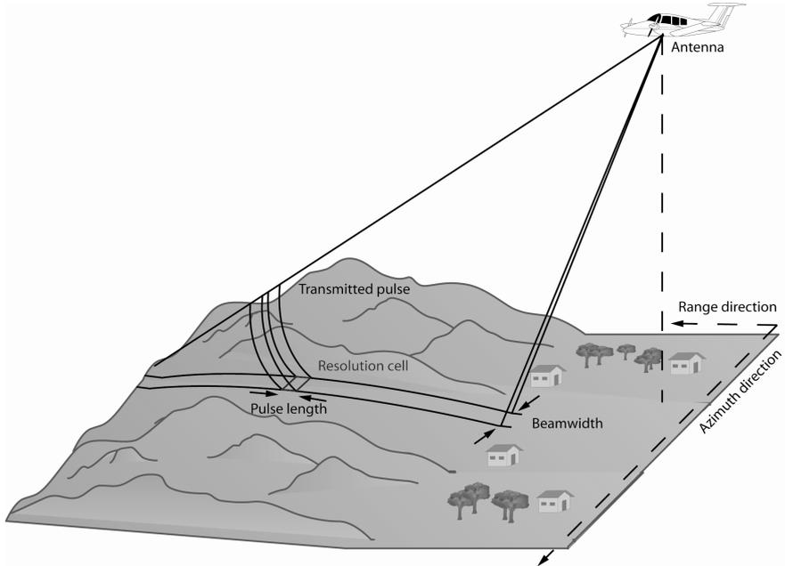
Figure 3-8. Geometry of a side-looking airborne RADAR system. Adapted from Lillesand and Kiefer (1987).
