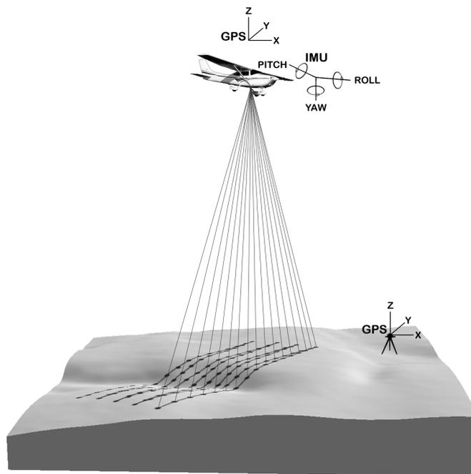
Figure 3-2. An illustration of airborne laser scanning.
