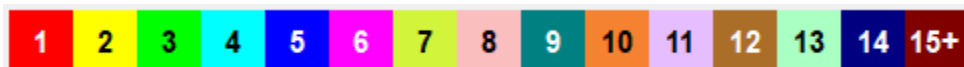
Figure 2. Colors used when coloring by return. Points labeled in data file as return 0 will be colored using the color for return 1.
