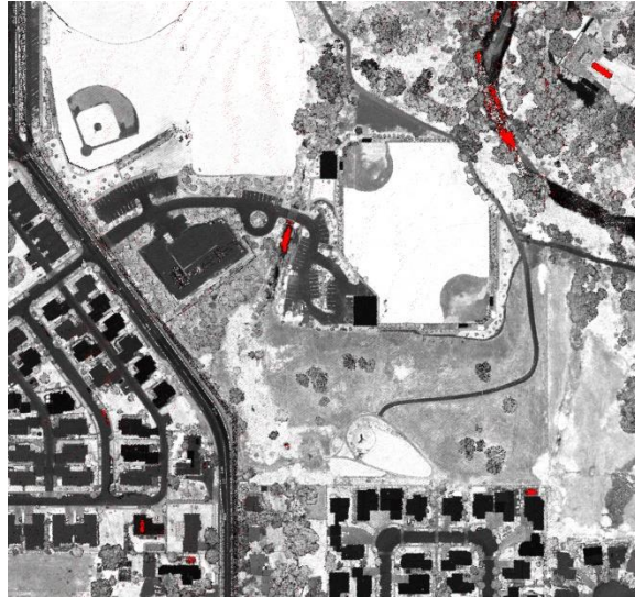
Figure 7. Final image produced using LIDAR intensity data for first returns. Red pixels in the image indicate areas where there were no first returns within the pixel. This image is the result of eight iterations using the grid origin offsets shown in figure 6. Image pixels are 0.30 by 0.30 m. Image represents an area that is 434 m wide and 411 m high.
