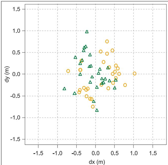
**Figure 7.** Horizontal error in lidar treetop measurement, narrow beam divergence setting. Green triangles denote Douglas-fir, and brown circles denote ponderosa pine. The mean positional error was 0.45 m (Douglas-fir), 0.56 m (ponderosa pine), and 0.50 m (all trees).
