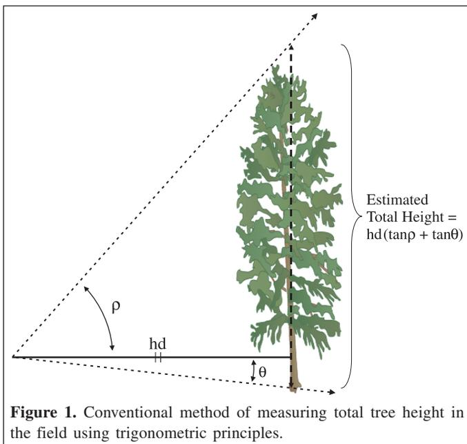
**Figure 1.** Conventional method of measuring total tree height in the field using trigonometric principles.
