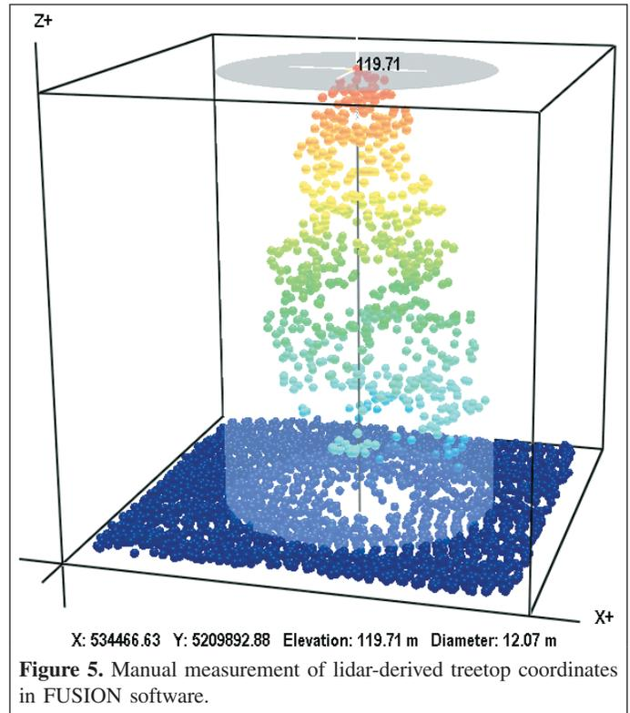
point cloud associated with each tree measured in the field can be isolated and displayed in a 3D perspective view (Figure 5).
