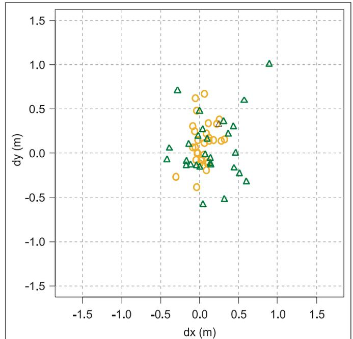
**Figure 8.** Horizontal error in lidar treetop measurement, wide beam divergence setting. Green triangles denote Douglas-fir, and brown circles denote ponderosa pine. The mean positional error was 0.40 m (Douglas-fir), 0.25 m (ponderosa pine), and 0.32 m (all trees).
