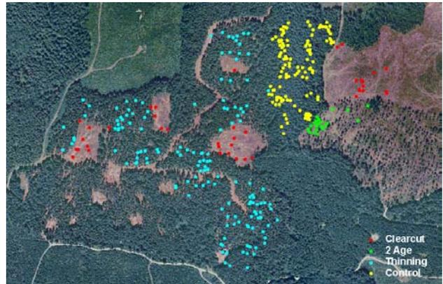
Survey checkpoints used to evaluate bare-earth surface model accuracy
