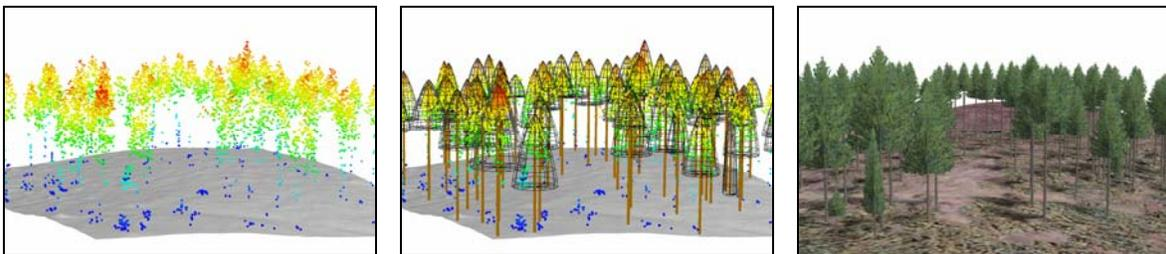
The lidar point cloud includes direct measurements of various canopy elements including stems, branches, and foliage. This series of images shows the lidar data for above-ground vegetation, tree objects inferred from these data, and a visual simulation of tree objects and terrain derived from lidar and rendered with PNW Research Station's EnVision software.
