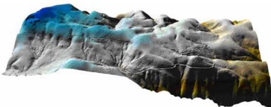
Bare-earth surface model created from lidar return data
