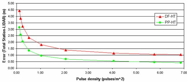
Error in Lidar-derived tree height measurements increases as the pulse density decreases.
